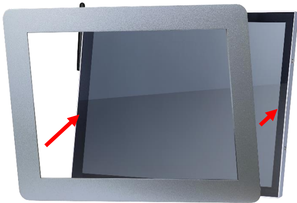
Step 1: Assemble the front module with the screen body. (This step is pre-assembled at the factory.)
