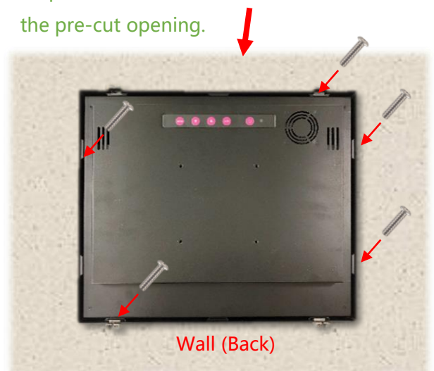
Step 3: Attach the clips from the back and secure with screws. (Up to 8 clips can be installed as needed or per positional limitations.)
