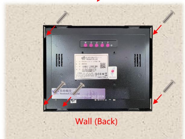
Step 3: Attach the clips from the back and secure with screws. (Up to 8 clips can be installed as needed or per positional limitations.)
