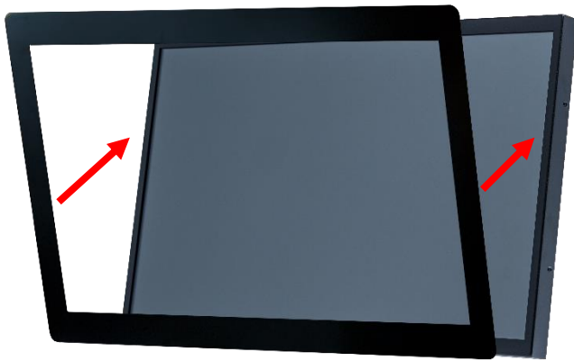
Step 1: Assemble the front module with the screen body. (This step is pre-assembled at the factory.)
