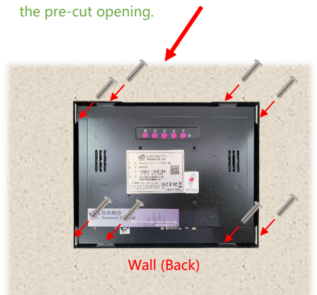
Step 3: Attach the clips from the back and secure with screws. (Up to 8 clips can be installed as needed or per positional limitations.)
